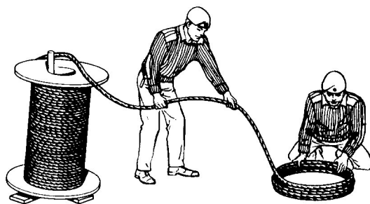
Fig 3-33. Lapping Off and Coiling Down a Small Wire Rope
