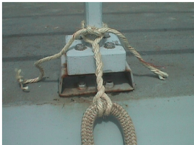
Fig 6-49(a). Correct Method of Rigging Hose Stops
