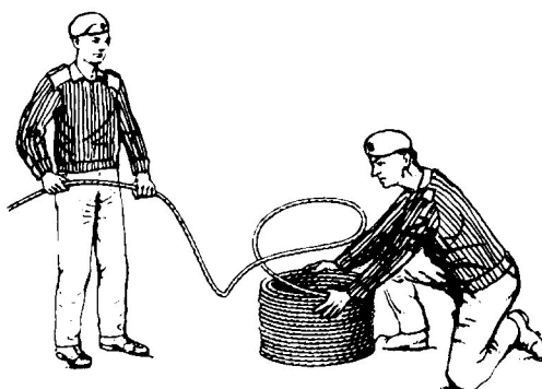
Fig 3-30. Running Out a Coiled Down Wire
